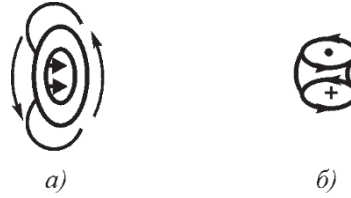
Fig. 8.1. Structure of a free electron: a - in metal; b - in free space
