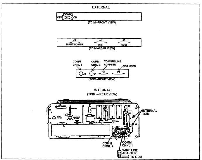
Figure 9-4. Wire and radio connections to the LCU
