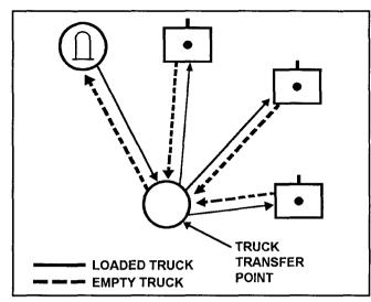
Figure 12-1. Double loop method of resupply
