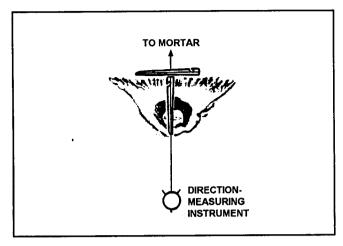
Figure J-6. Splinter groove method
