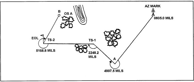
Figure 5-7. Example of a directional traverse
