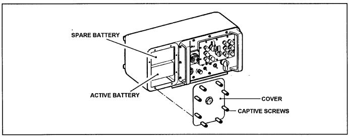
Figure L-10. Battery installation in the case assembly
