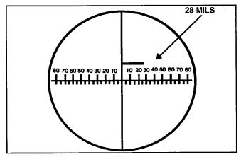
Figure D-2. Aiming post sight picture at 50 meters
