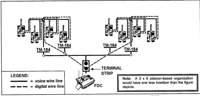
Figure 9-9. Positioning for platoon-based battery using one BCS
