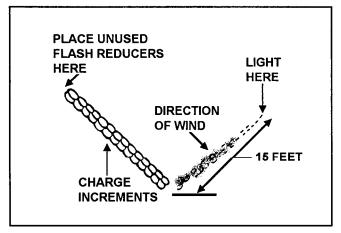
Figure 10-3. Layout for burning powder increments
