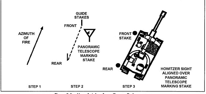
Figure 2-5. Use of stakes for self-propelled weapons
