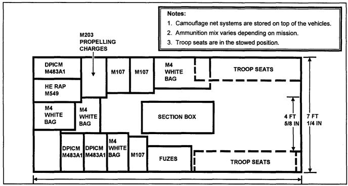
Figure E-1. Example 5-ton prime mover load plan for M198 section
