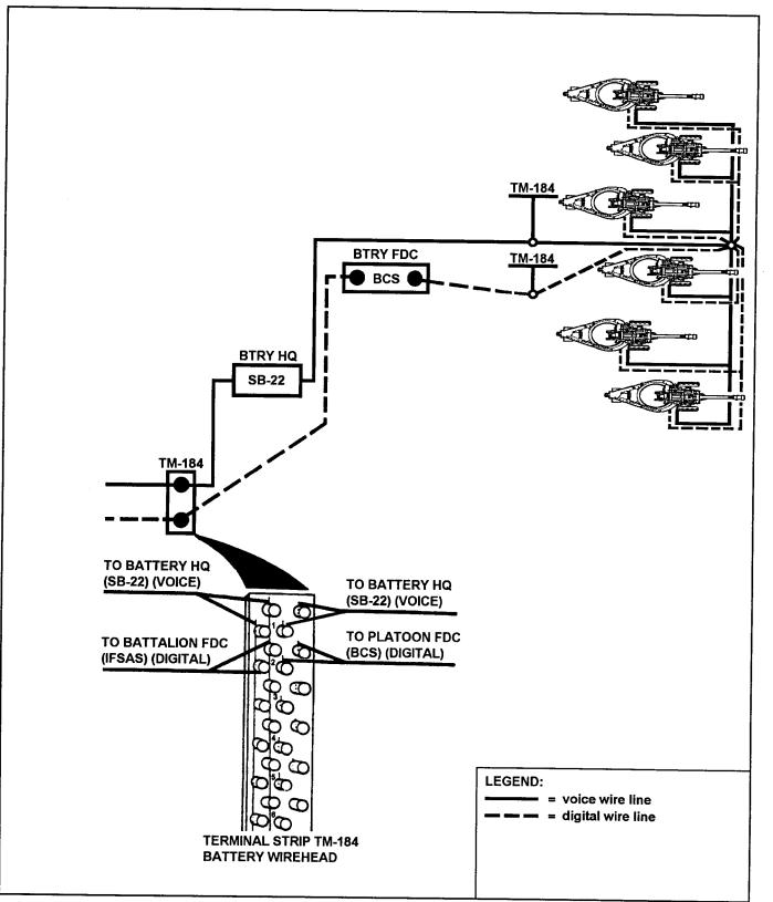
Figure 9-6. Battery-based battery wire system
