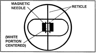
Figure 4-7. Centering the magnetic needle
