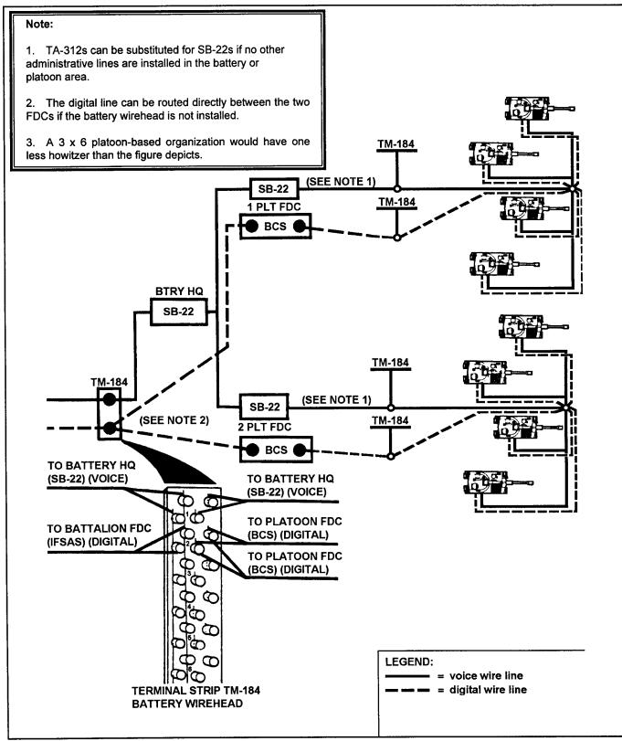
Figure 9-5. Platoon-based battery wire system
