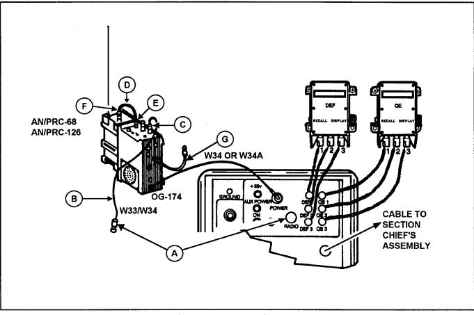
Figure L-16. Gun section cabling for howitzer sections
