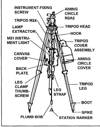
Figure 4-4. Aiming circle with tripod
