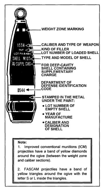
Figure 10-2. Markings of a (separate-loading) projectile
