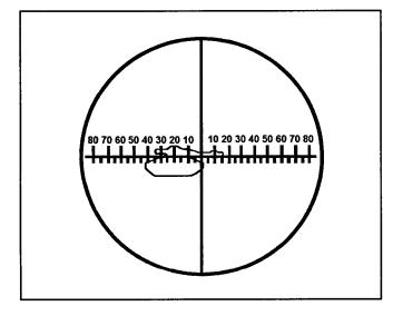
Figure 8-1. Gunner's sight picture, reticle laying (lead R20)
