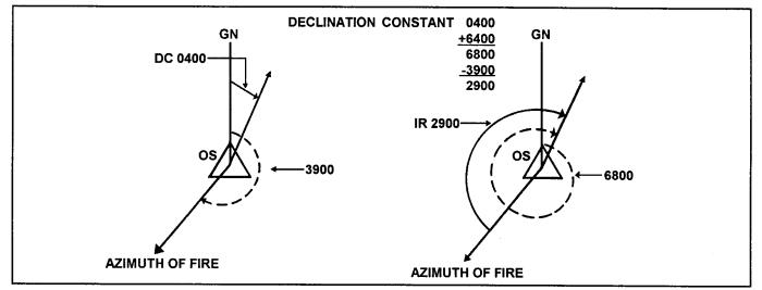
Figure 4-16. Computation of instrument reading
