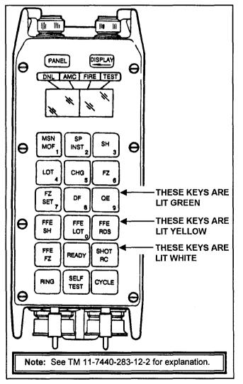
Figure L-2. Section chief's assembly controls, indicators, and connectors
