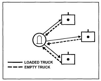
Figure 12-2. Single loop method of resupply
