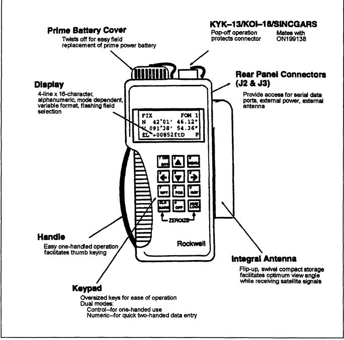
Figure 4-8. Precision lightweight GPS receiver (PLGR)
