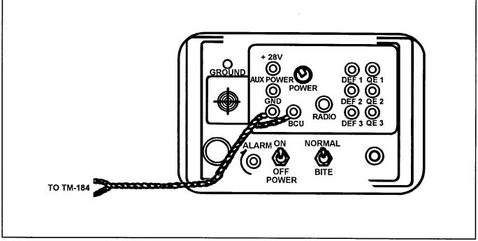
Figure 9-3. Wire line connection to the GDU
