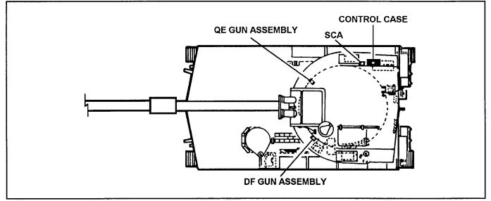
Figure L-9. GDU location on an M109-series howitzer
