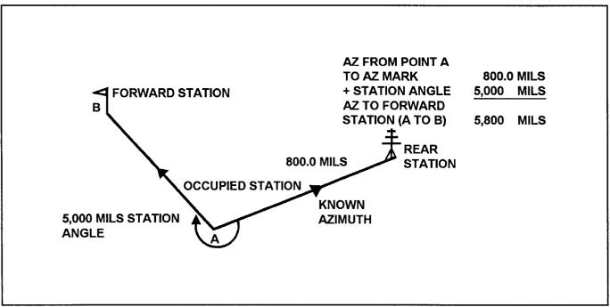
Figure 5-6. Fieldwork requirements for directional traverse
