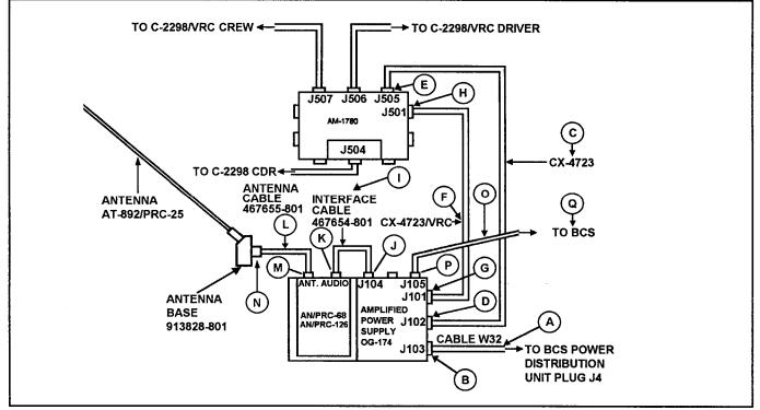
Figure L-15. FDC cabling for the AN/PRC-68 or AN/PRC-126
