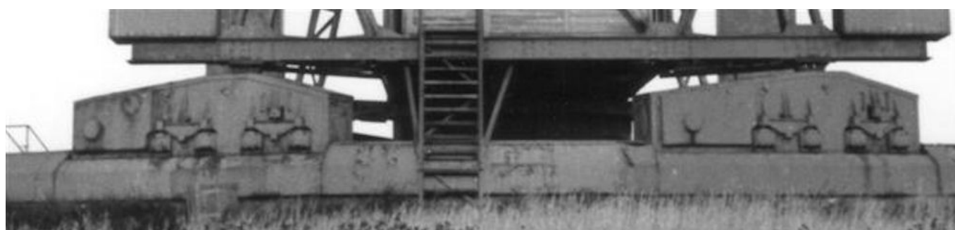
Fig. 63 Each locomotive has two bogies (Be-10 at Hundborg) - 32 wheels in total (source: www.gyges.dk , used with permission)
