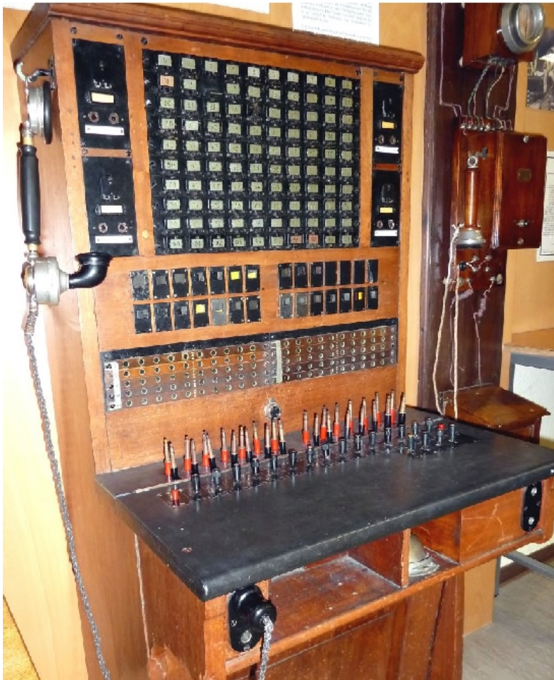
Fig. 170: Left "Klappenschrank" telephone switchboard model OB-14; right: 50-line Wehrmacht PBX
