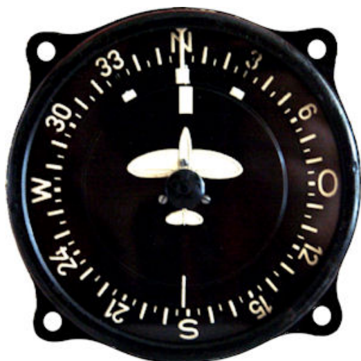
Fig. 152: Remote compass, as used in Fw190 etc.
