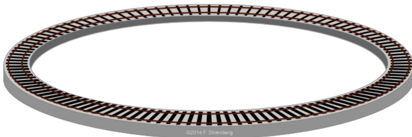
Fig.2: Concrete ring with the circular rail track
