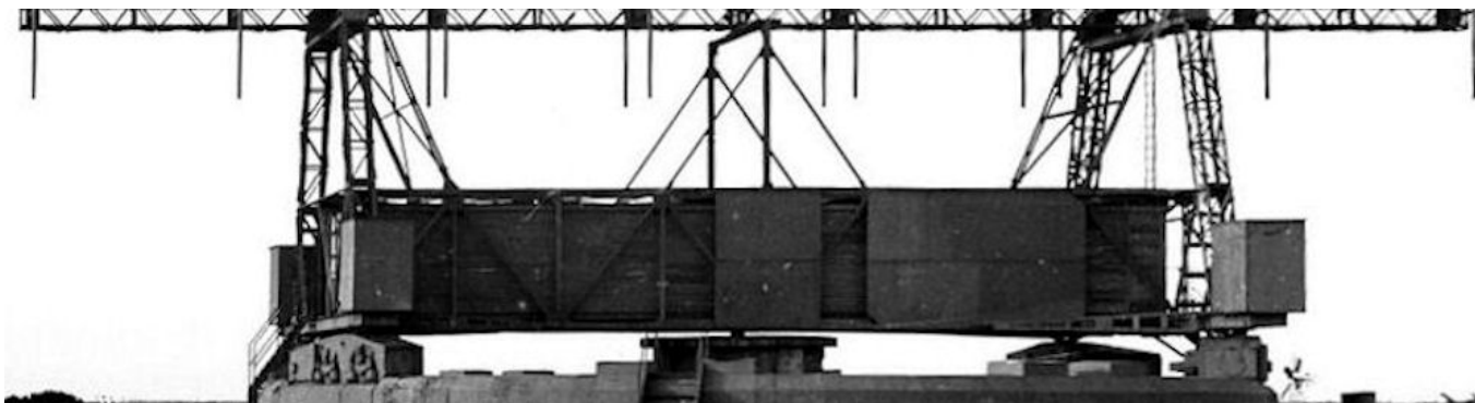
Fig. 52: The cabin at Be-10 Hundborg/Denmark - with protective siding panels
