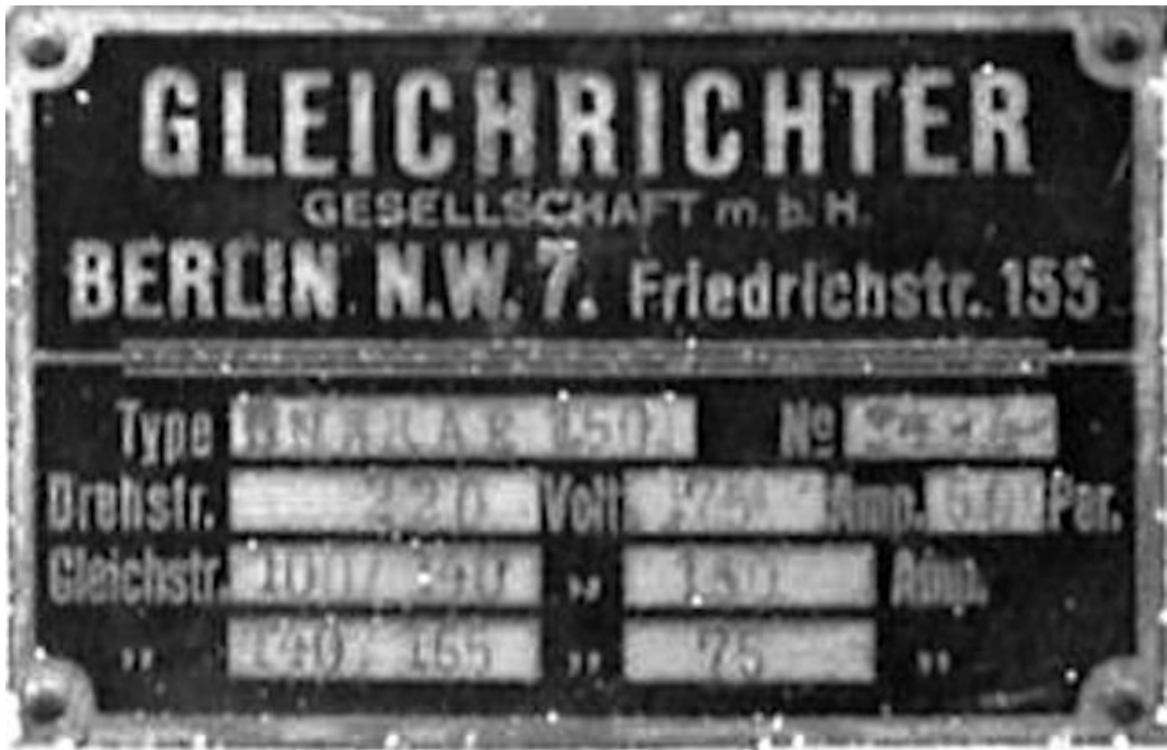
Fig. 89: Label of a BBC MAR-cubicle with a MAR built by Gleichrichter G.m.b.H. in Berlin (source: H.-T. Schmidt homepage ; MAR for 220 volt 3-phase AC @ 75 amps, 100/140 volt DC @ 150 amps, 140/165 volt DC @ 65 amps)
