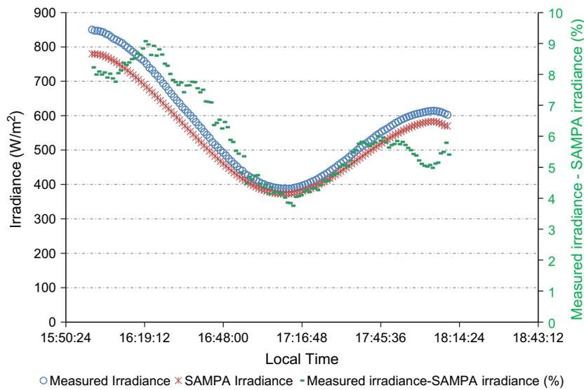
Fig. 5. Measured irradiance versus calculated irradiance using SAMPA during the June 10, 2002 partial solar eclipse.
