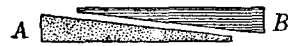
FIG. 79. for example, in Fig. 79, A is a wedge of quartz whose crystallographic axis is parallel to the edge of the wedge, while B is another plate
