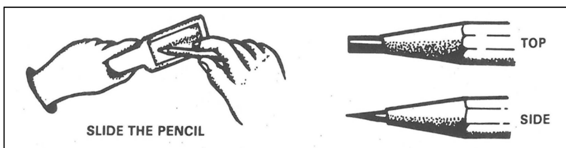
Figure 6-2. The 6H Pencil (Wedge Point).
