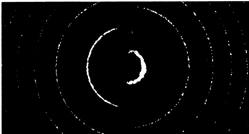
Fig. 2. Fabry-Perot interferograms of incident and backscattered phase-conjugate (Brillouin-shifted) beams. [After Zel'dovich et al. (1972).]
