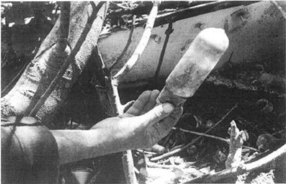
Mercury-toxic radio tube (model 872A rectifier) found in dump
