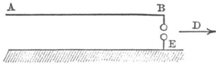
FIG. 210. Marconi's directive antenna.
