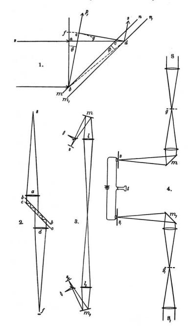
would be about one-millionth of the original intensity, so that if sunlight or the electric arc were used it could still be readily seen. The mirrors *bb*, and *cc*, would differ from parallelism sufficiently to separate the successive images. Finally, the apparatus need not be mounted so as to revolve, as the earth's rotation would be sufficient.
