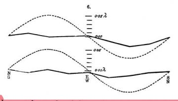
placement due to the relative motion of the earth and the luminiferous ether, this cannot be much greater than 0.01 of the distance between the fringes.
