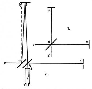
and ca is partly reflected along ad. If then the paths ab and ac are equal, the two rays interfere along ad. Suppose now, the ether being at rest, that the whole apparatus moves in the direction sc, with the velocity of the earth in its orbit, the direction sc are equal to be appreciated at the second second
