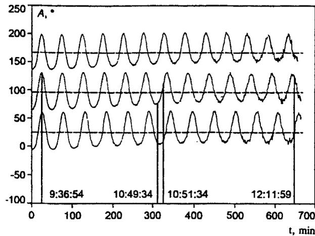
Fig. 2. Azimuth of oscillation plane as a function of time for the second pendulum.
