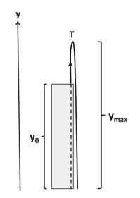
Figure 1.2 From the top of a building of height  $y_0 = 15m$ , I throw a rock with an initial upward velocity of  $v_0 = 10m/s$ . The dotted line represents the trajectory continued back to earlier times.
