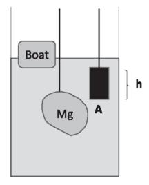
Figure 20.6 The irregular object of mass *M* displaces a volume of liquid equal to its own. The loss in its weight is the weight of that body of liquid. This is more readily seen for a regular object like the cylinder shown to the right. At the top left is a boat whose weight equals the weight of the liquid displaced by the fraction immersed.
