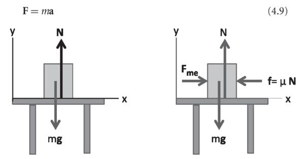
Figure 4.2 A mass *m* sitting on a table, (left) without and (right) with friction. The coefficient  $\mu = \mu_S$  if the block is at rest and  $\mu = \mu_k$  if it is moving.
