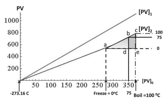
Figure 21.3 Comparison of different gas thermometers labeled 0, 1, and 2. The *x*-axis is labeled by one and the other two correspond to two other gas thermometers, possibly filled with different dilute gases. The linearity of the graphs guarantees that the thermometers will agree not only at 0 and 100, where they have to, but also everywhere in between given the similarity of triangles *abd* and *ace*. When  $[PV]_0 = 350$ , the temperature is 75°C.
