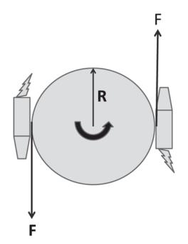
Figure 10.3 A rocket-powered merry-go-round of mass *M*. Each engine has a thrust *F*, mass *m*, and contributes  $mR^2$  to the moment of inertia.
