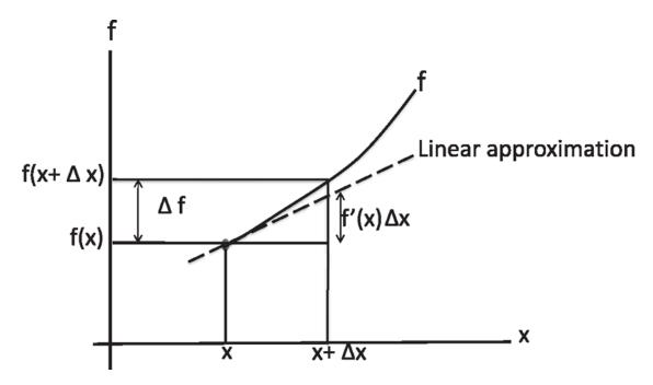
Figure 6.1 The change,  $\Delta f$ , in a function f(x) as x changes by  $\Delta x$ , may be approximated by  $\Delta f \simeq f(x)\Delta x$ , where  $f'(x) = \frac{df}{dx}$ . The solid line is the actual function and the dotted line is the approximation by a straight line of slope f(x).
