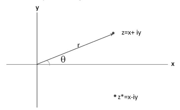
Figure 16.2 The complex plane with a typical point z = x + iy and its conjugate  $z^* = x - iy$ . In polar form, z is assigned a length r and an angle  $\theta$ . We will see that  $z = re^{i\theta}$ . Note that we measure y and not iy along the y-axis.
