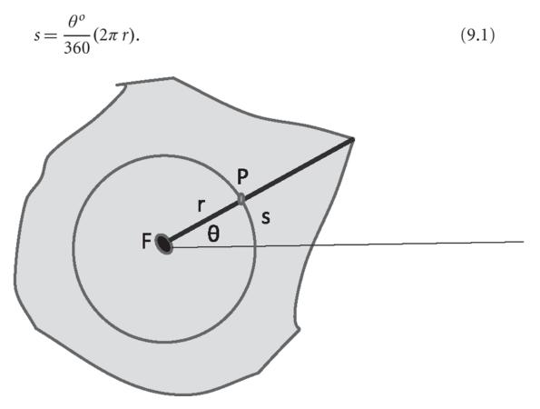
Figure 9.2 As the rigid body rotates around some fixed point F, a typical point P at a distance r from F moves on a circle of radius r.
