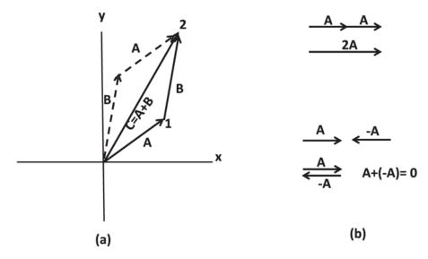
Figure 2.2 Adding vectors. Part (a) shows how to add vectors and that  $\mathbf{A} + \mathbf{B} = \mathbf{B} + \mathbf{A}$ . Part (b) illustrates the meaning of multiplying a vector by a number (2 in this example) and the null vector **0**.
