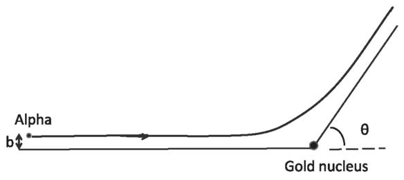
Figure 8.10 An alpha particle approaching a gold nucleus with impact parameter *b*. If you assume the nucleus is immobile and exerts a Coulomb force  $1/r^2$ , you can calculate the direction  $\theta$  in which the alpha particle will emerge, as a function of *b* and the energy. If a beam of particles with a distribution of *b*'s is given, one can predict the particle flux in any direction  $\theta$ .
