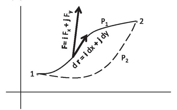
Figure 6.3 The line integral of a force between points 1 and 2 along a path  $P_1$  is the sum of dot products  $\mathbf{F} \cdot d\mathbf{r}$  over tiny segments that make up the path, in the limit  $d\mathbf{r} \rightarrow \mathbf{0}$ . Also shown by a dotted line is another path  $P_2$  between the same end points.
