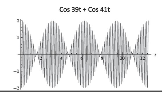
Figure 19.3 Beats due to two waves of unit amplitude A = 1 and large but nearly equal angular frequencies  $\omega_1 = 41$ ,  $\omega_2 = 39$ . The (angular) beat frequency is supposed to be  $\omega_b = 41-39$  rads/s, which means a time  $T = \frac{2\pi}{\omega_b} = \pi$  between beats, in accord with the figure.
