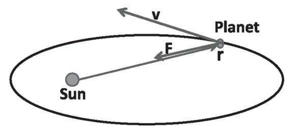
Figure 3.2 The planet is separated from the sun by **r**. The force **F** on it was determined to be always opposite to **r**, i.e., pointing toward the sun and falling as  $\frac{1}{r^2}$ . (The force is slightly offset from **r** for clarity.)
