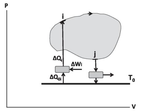
Figure 24.1 A system is taken quasi-statically through a cycle. In the segment labeled *i* it needs some heat  $\Delta Q_i$ , which it gets from a Carnot refrigerator operating between the system's current temperature and a reservoir at  $T_0$ . The refrigerator needs work  $\Delta W_i$ . If it happens that  $\Delta Q_i < 0$ , as is the case at point *j*, the heat will be sucked out of the system by a Carnot engine and dumped into the reservoir at  $T_0$ .
