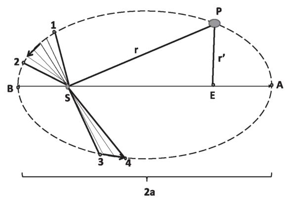
Figure 7.1 The solar system seen from afar, with just one planet *P* shown. The orbit is an ellipse with the sun *S* at one focal point, and a major axis 2a that obeys r + r' = 2a. The position vector sweeps out equal areas in equal times, for example, between 1 and 2 and between 3 and 4.
