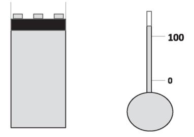
Figure 21.1 Left: The gas is inside the cylinder capped by a piston of area *A*. The weights on the piston exert a force *F* and pressure  $\frac{F}{A}$ . Right: A thermometer with a liquid that expands from the bulb into the thin calibrated stem.
