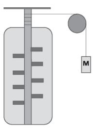
Figure 21.7 Joule's experiment to find the mechanical equivalent of heat, 4.2kJ/kcal. As the weight descends, the fins turn and heat up the water. The missing mechanical energy in the weight becomes heat energy. (It is assumed that the rest of the apparatus does not absorb any appreciable part of the generated heat.)
