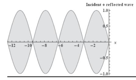
Figure 19.7 Nodes and anti-nodes on a string with A = 0.5 and k = 1 or  $\lambda = 2\pi$ . The incoming and reflected waves form a *standing wave*, with nodes at  $0, -\pi, -2\pi, \ldots$  and anti-nodes at  $-\frac{\pi}{2}, -\frac{3\pi}{2}, \ldots$ . The vibrating string is a blur, shown by the shaded region.
