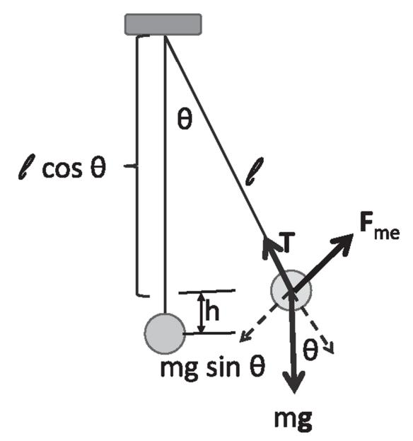
Figure 9.5 A pendulum made up of a massless string length *l* and a bob of mass *m*. The force *m***g** is resolved in the radial and tangential directions. The bob has climbed up a height  $h = l - l \cos\theta$ .
