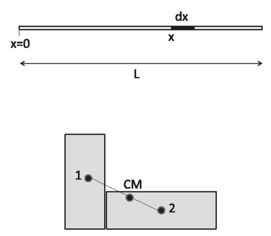
Figure 8.3 (Top) A rod of length *L* and mass *M*. (Bottom) An L-shaped object made of two rectangles. The points 1 and 2 are the CMs where all their mass may be assumed to be concentrated. The point marked CM is the weighted sum of 1 and 2.
