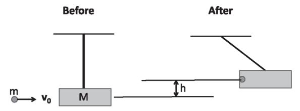
Figure 8.9 A bullet of mass *m* and velocity  $\mathbf{v}_0$  plows into a suspended block of wood of mass *M*, and the two of them rise as a pendulum to height *h*.
