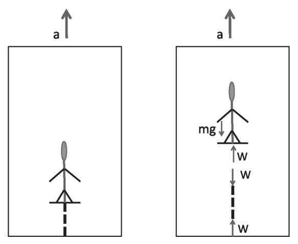
Figure 3.5 (Left) An elevator is accelerating at a rate *a* and you are standing on a scale whose spring is shown by a dotted line. (Right) The free-body diagram for you and the spring. The spring is compressed at each end by a force *W*.
