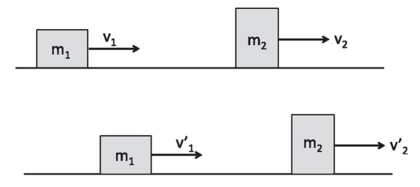
Figure 8.8 (Top) A body of mass  $m_1$  and velocity  $v_1$  collides with a body of mass  $m_2$  and velocity  $v_2$ , with all velocities shown as positive. (Bottom) The two bodies with final velocities  $v'_1$  and  $v'_2$ .
