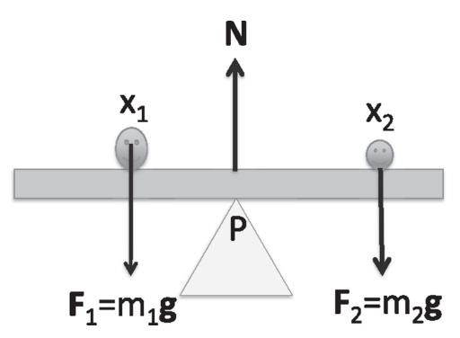
Figure 11.1 Two kids on a seesaw. The supporting pivot provides a force **N** upward. The total torque due to the kids' weights  $\mathbf{F}_1 = m_1 \mathbf{g}$ ,  $\mathbf{F}_2 = m_2 \mathbf{g}$  and the pivot force **N** is zero.
