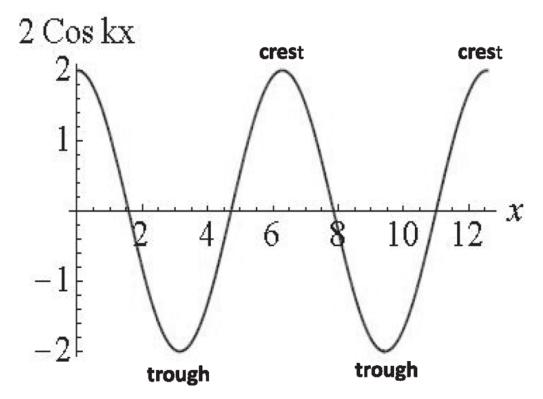
Figure 18.3 The wave  $A \cos(kx - \omega t)$  at t = 0 as a function of x for the choice A = 2, k = 1. For k = 1,  $\lambda$  should be  $2\pi \simeq 6.28$  according to Eqn. 18.29, and indeed it is. The maxima are called *crests* and the minima are called *troughs*.
