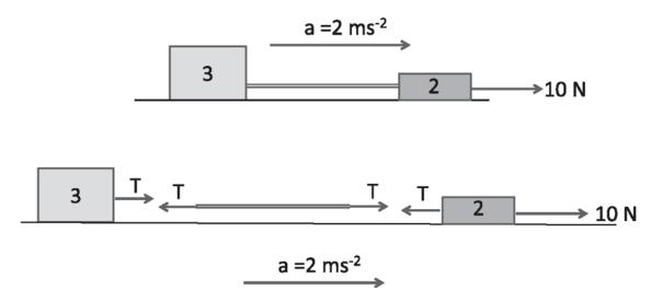
Figure 3.4 (Top) A force of 10 N pulls the two blocks connected by a massless rope, all treated as a single entity. (Bottom) The free-body diagram for the two blocks and the rope, which experiences equal and opposite forces of magnitude T called the tension.
