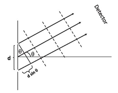
Figure 19.5 Computing the path difference in the double-slit experiment when the detector is very far from the slits. The dotted lines are the troughs.
