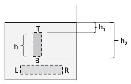
Figure 20.2 The horizontal dotted cylinder marks a part of the fluid in equilibrium under forces from the left L and right R. The vertical dotted cylinder marks a part of the fluid in equilibrium under forces from the top T and bottom B and its weight Mg.
