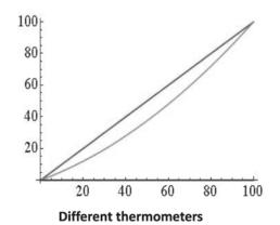
Figure 21.2 The *x*-axis is labeled by the reading of a reference thermometer, say with mercury. Along the *y*-axis are plotted the readings as per another—say, an alcohol—thermometer (curved line) along with a straight line y = x, which is just the reading of the same mercury thermometer plotted for easy comparison.
