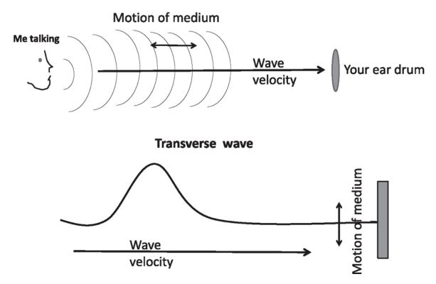
Figure 18.1 Top: A sound wave is longitudinal: the sound goes from left to right and the air also vibrates back and forth. Bottom: The wave on a string is transverse: the wave goes from left to right, but the string moves up and down.
