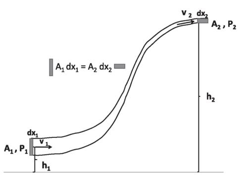
Figure 20.7 The flow of a fluid along a pipe of varying cross section, pressure, and height. We focus on the part initially between cross-sectional areas  $A_1$  and  $A_2$ . In a time dt, it is left unchanged but for a sliver of volume  $A_1dx_1 = A_1v_1dt$ , which has been removed from the left and appended to the right end as a sliver of equal volume  $A_2dx_2 = A_2v_2dt$ .
