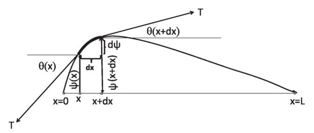
Figure 18.2 The string under tension *T* has mass  $\mu$  per unit length and is fixed at x = 0 and x = L. The highlighted segment has a width dx, with the same tension *T* pulling the two ends but at slightly different angles. The displacement  $\psi$  and angles  $\theta$  are exaggerated for clarity. The derivation is valid only when all these are very small.
