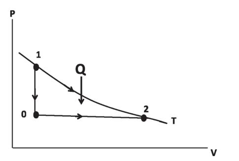
Figure 24.2 The entropy change between 1 and 2 at the same *T* can be computed by integrating  $\frac{dQ}{T}$  along the isotherm or any other path, such as the one that goes via point 0.
