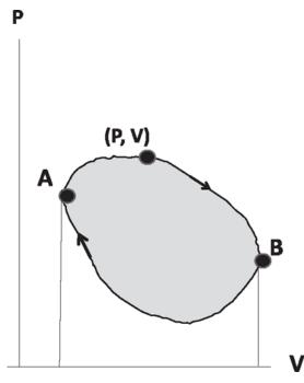
Figure 23.1 The work done by a gas as it goes over a closed cycle equals the area enclosed by the cycle in the P - V plane. During *AB* the gas expands and does work, and during *BA* it is compressed and has work done on it. The shaded area is the algebraic sum of the two.
