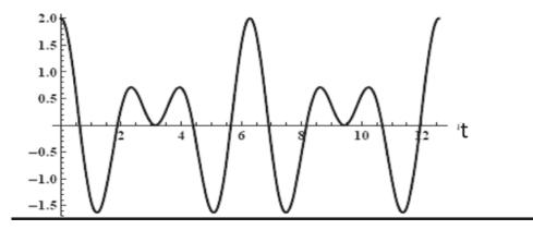
Figure 19.2 Superposition of two waves of unit amplitude A = 1 and angular frequencies  $\omega_1 = 2$ , and  $\omega_2 = 3$ . At t = 0 they are in step, at  $t = \pi$  their phases differ by  $\pi$  and they cancel, at  $t = 2\pi$  they are in step, and this repeats every  $2\pi$  seconds.
