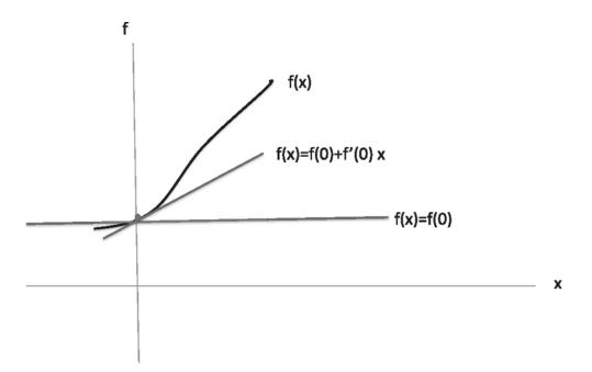
Figure 16.1 A sample function f(x) and two approximations to it near x = 0 based on the Taylor series. The flat line f(x) = f(0) assumes f(x) does not change as we move away from x = 0. It is based on the first term in what is called the Taylor series. The second line f(x) = f(0) + f'(0)x is the linear approximation based on two terms, and it matches the function and its derivative at x = 0. It assumes the slope does not change.
