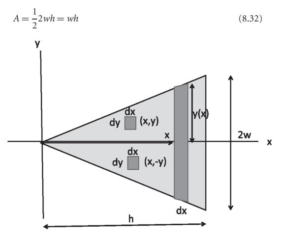
Figure 8.4 The CM calculation of a triangle of base 2w and height *h*. It is viewed as a weighted sum over rods of width dx and height 2y(x).
