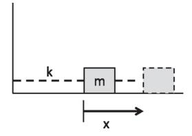
Figure 17.1 The mass m rests on a table and is connected to a spring of force constant k, which is anchored to the wall. The displacement from equilibrium is denoted by x. It is positive in the figure but it could also be negative if the mass were to be displaced the other way.
