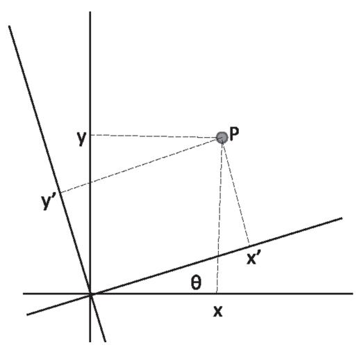
Figure 13.1 The same point P (solid dot) is assigned coordinates (x,y) by me and (x',y') by you. The pairs of coordinates are linearly related. The dotted lines indicate the sizes of the coordinates in the two frames.
