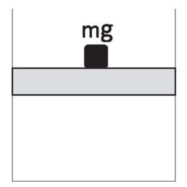
Figure 20.1 A gas in a cylinder with a massless piston of area *A* on top. The mass *m* exerts a force *F* = mg and a pressure  $P = \frac{mg}{A}$  Pascals.
