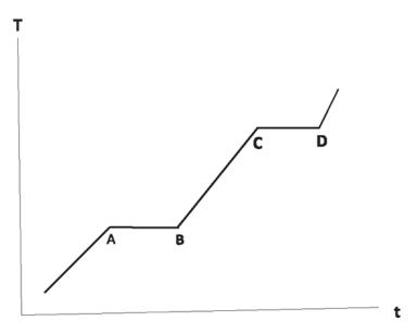
Figure 21.5 Different phases of water from ice below  $0^{\circ}C$  to water above  $100^{\circ}C$ . As time *t* increases, a steady flow of calories first heats the ice below  $0^{\circ}C$  to *A*, where it melts *at*  $0^{\circ}C$  between *A* and *B*. The water then heats up between *B* and *C*, and then it evaporates *at*  $100^{\circ}C$  between *C* and *D*, before becoming superheated steam.
