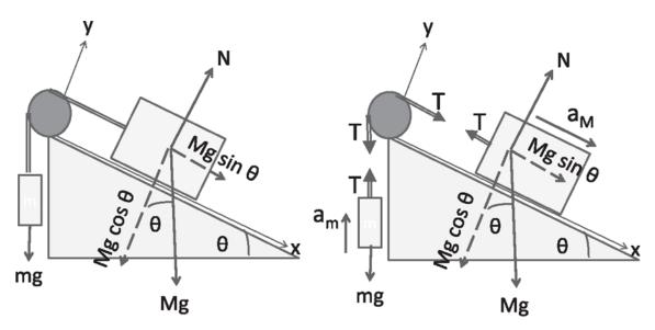
Figure 4.4 (Left) Two masses linked by a massless rope and massless pulley. (Right) The free-body diagram.
