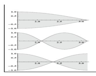
Figure 19.9 From the top: First two modes of vibration of a tube of length  $\pi$  closed at the right end and open at the left end followed by the first mode of a tube of length  $\pi$  open at both ends. You can read off the  $\lambda$ 's by inspection and deduce the frequencies from  $v = \lambda f$ .
