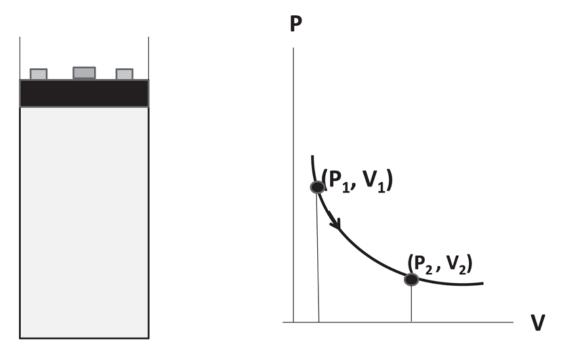
Figure 22.3 Left: A piston and cylinder combination. The weights balance the pressure *P* of the gas inside. (The atmospheric pressure is assumed to be zero or added to that of the weights.) The volume *V* is just the volume below the piston. Right: A point  $(P_1, V_1)$  representing a state of the gas and a possible quasi-static path in the *P* –*V* plane to state  $(P_2, V_2)$ . To move quasi-statically, the weights must be replaced by fine grains of sand, which may be added or removed.
