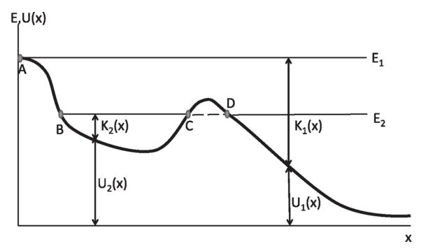
Figure 6.5 The roller-coaster ride. The total energy is fixed at  $E_1$  or  $E_2$  in the two examples discussed. At every point *x*, the sum of the potential energy U(x) and the kinetic energy K(x) equals a constant *E*. If the energy is  $E_2$ , the coaster can only be found between *B* and *C* or to the right of *D*. It is disallowed in the region *CD* where the potential energy exceeds the total energy, and *K* would have to be negative.
