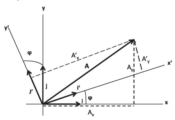
Figure 2.4 The same vector **A** is written as  $\mathbf{i}A_x + \mathbf{j}A_y$  in one frame and as  $\mathbf{i}'A'_x + \mathbf{j}'A'_y$  in the other. The dotted lines indicate the components in the two frames.
