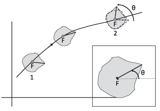
Figure 9.1 A rigid planar body undergoing translation and rotation in a plane as it goes from state 1 to state 2. The dot represents the fixed point *F*. The solid line from the *F* to the pointy edge of the object allows us to follow its rotation. In state 2 the original orientation is shown in dotted lines and the curved arrow shows the rotation  $\theta$  needed to bring it to the final orientation.
