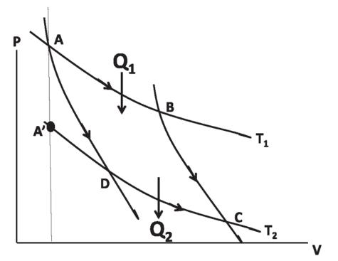
Figure 23.2 The figure shows two isothermal curves at  $T_1$  and  $T_2$  and two adiabatic curves crossing them. In the latter case *P* falls more rapidly with increasing *V* because it gets no help from outside.
