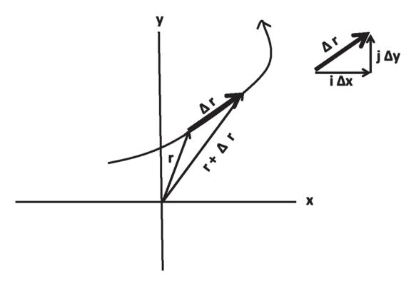
Figure 2.5 The particle moving along some curved path goes from **r** at time *t* to  $\mathbf{r} + \Delta \mathbf{r}$  at time  $t + \Delta t$ . The velocity **v** is the limit of the ratio  $\frac{\Delta \mathbf{r}}{\Delta t}$  as  $\Delta t \rightarrow 0$ , and thus parallel to  $\Delta \mathbf{r}$ , which eventually becomes tangent to the curve.
