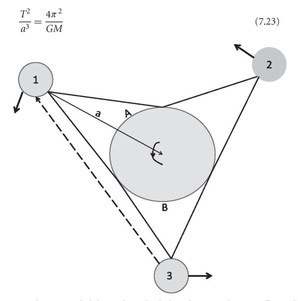
Figure 7.2 The view as we look down at the North Pole shows three geosynchronous satellites, each of which hovers over a fixed point on the earth, takes 24 hours per revolution, and covers a part of the earth as shown. By communicating with them, and allowing them to communicate with each other, any point on the earth can communicate with any other. If *B* can send the image of a game to satellite 3, it can send it to 1 along the dotted line, and that in turn can beam it to me at *A*.
