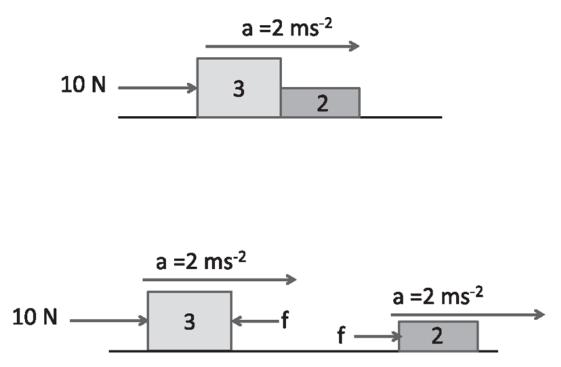
Figure 3.3 Top: A force of 10 *N* acts on the two blocks, viewed as a single entity. Bottom: The freebody diagram for the two blocks showing all the forces *on* each block. Notice the third law is being invoked.
