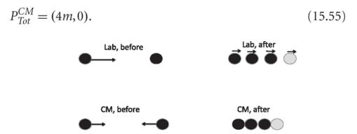
Figure 15.2 Top: The collision of a projectile proton and a static target proton, leading to three protons and an antiproton produced with the minimum energy. The final four particles cannot be at rest in the lab frame due to momentum conservation. Bottom: The minimal collision as seen in the CM frame, where the final four particles are allowed to be at rest.
