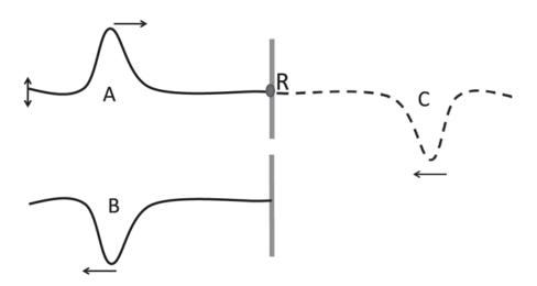
Figure 19.6 Part A: The blip I generate (up-and-down arrow at left) goes to the wall at the right (solid vertical line). Part B: The blip gets reflected from the wall at point *R*, reversed in direction and in sign. Part C: There is no wall, but a blip comes from the right and cancels the original blip at the wall for all times. The former keeps moving to the left and becomes the reflected blip of part B.
