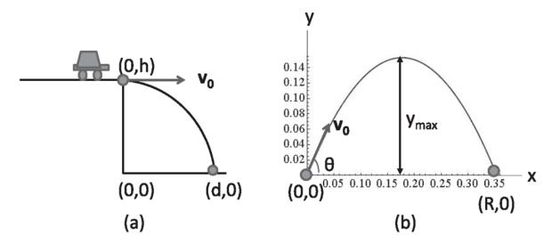
Figure 2.8 (a) A car flies off the cliff at (0,*h*) and lands at (*d*,0). (b) A projectile is launched with initial velocity  $\mathbf{v}_0 = (\mathbf{i} + \sqrt{3}\mathbf{j})m/s$  The range is R = 0.35 m and the maximum height reached is  $y_{max} = 0.15 m$ .
