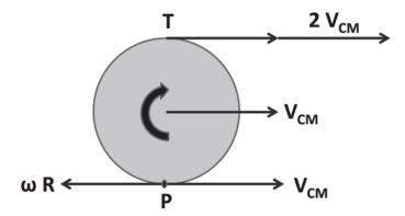
Figure 10.2 A tire of radius *R* that is rolling clockwise at  $\omega$  without slipping. At the contact point *P*, the CM velocity  $\mathbf{V}_{CM}$  cancels the tangential velocity  $\omega R$ , while at the top, *T*, it doubles it. The point *P* is instantaneously at rest with respect to the road.
