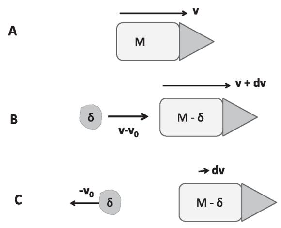
Figure 8.7 (A) The rocket at time *t* as seen from the ground. (B) The rocket at time t + dt as seen from the ground. It has lost mass  $\delta$  in the form of emitted gases and gained speed *dv*. The fumes of mass  $\delta$  (the blob) are moving at a speed ( $v - v_0$ ) relative to the ground. (C) The rocket and fumes at time t + dt in the frame moving at velocity v(t). The fumes have an exhaust velocity  $- v_0$  in the rocket frame.
